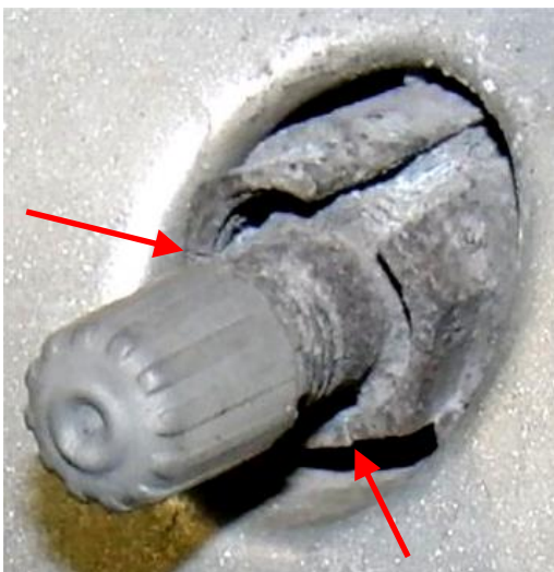
Figure 5: Split stem nut on left rear.
