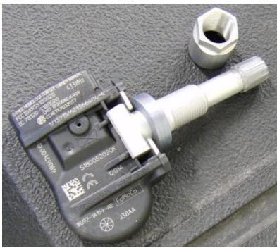
Figure 1: Exemplar TPMS unit, with stem nut removed.
