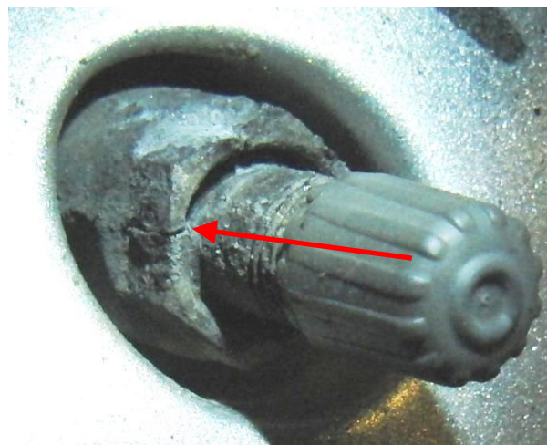
Figure 6: Fracture on right rear stem nut
