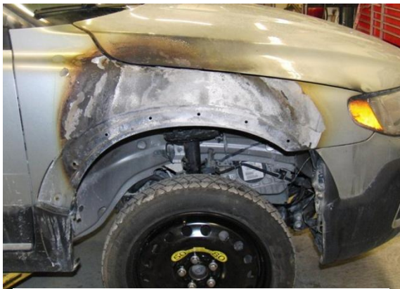
Figure 3: Burn pattern on fender.
