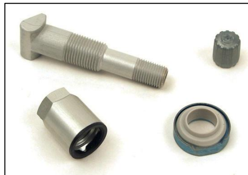
Figure 2: Typical TPMS service kit components.
