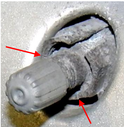
Figure 5: Split stem nut on left rear.
